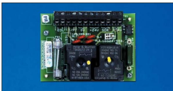
The SB520 enables the SNM800 to drive sounder circuits with higher currents whilst maintaining the reverse polarity integrity line monitoring.
