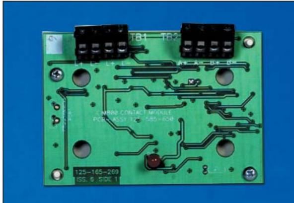
The CIM800 is a flexible addressable input-monitoring device that fits in the standard ancillary housings.
