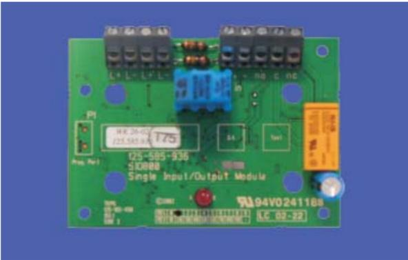
The SIO800 is designed to provide a monitored input and a volt free relay changeover output. It consists of an input for monitoring the status of a normally open contact and output changeover relay contact. The relay is controlled by a command sent from the MX Fire Controller via the addressable loop.
