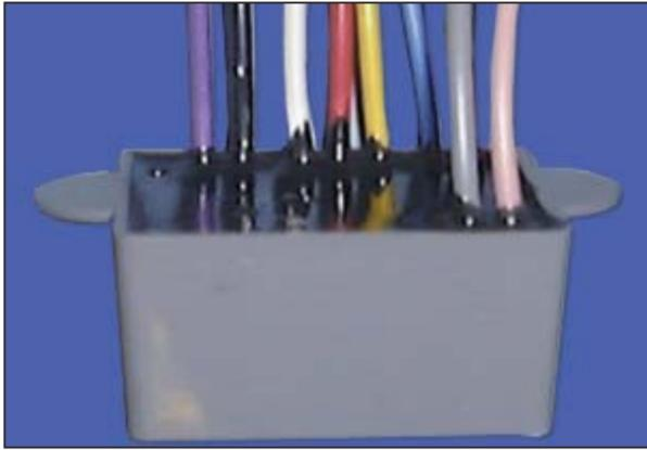
The HVR800 is a non-addressable device which allows a low current mains rated relay to switch up to 10A. Alternatively a low voltage drive signal such as that provided by the RIM800 or 80 way mimic can be used to switch the integral mains relay.
