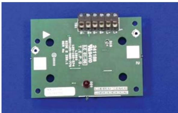
The LI800 is designed to be used on all MX addressable loops. It monitors the line condition and upon detection of a short circuit it isolates the affected section whilst allowing the rest of the addressable loop to function normally.
