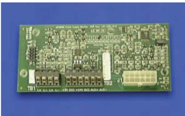
The APM800 is an MX addressable power supply monitoring module which is usually used with the PSM800 power supply module to make an addressable power supply. The APM800 is designed to fix to studs on the top of the PSM800. The APM800 monitors the PSM800 for mains failure, earth fault, battery charger fault and battery fault. It can reset the PSM800 resettable 24Vd.c. output and initiate a battery test which then reports battery voltage and current to the controller.
