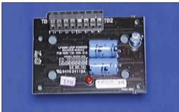
The LPS800 provides a single monitored sounder output circuit with up to 75mA of power sourced from the MX panel loop.
