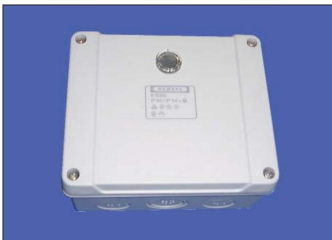
The D800 Ancillary Housing is a surface mount IP55 plastic housing which will accommodate any one of the 800 module range except for the APM800/MIM800/TM520.
