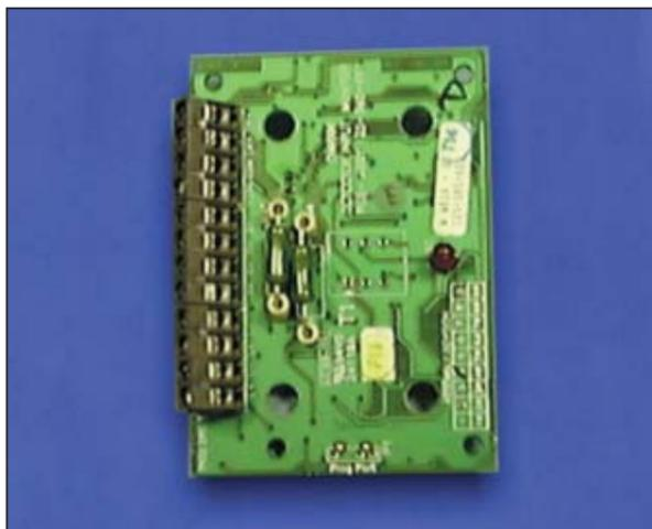
The DIM800 is designed to power and monitor a circuit of low voltage conventional detectors and callpoints. The detection circuit is powered from an external 24V d.c. supply and is reset by the MX addressable panel. The DIM800 monitors the external 24V d.c. and provides a fault signal if it is lost. The input detection circuit can be wired as one or two spur circuits (Class B), one loop configured circuit (Class A) or one 4 wire detection circuit.
