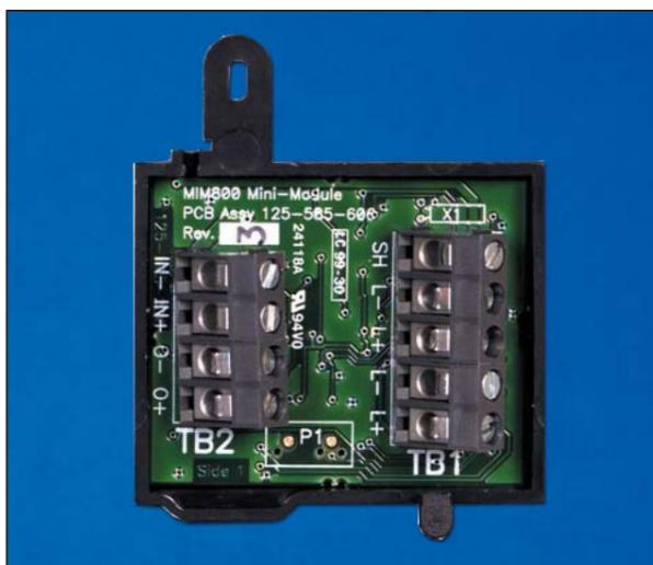
The MIM800 is a small MX addressable module designed for monitoring a single input circuit. The MIM800 can monitor normally open or normally closed inputs and provides open and short circuit monitoring of the line.
