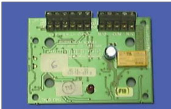
The RIM800 provides a single programmable relay output from the MX DIGITAL addressable loop which can be programmed for a variety of applications including signalling fire conditions to plant, machinery, fire doors, dampers & security systems.
