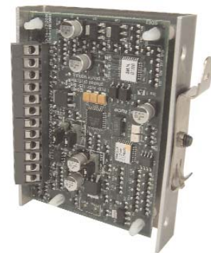
DDM800 Module on DIN rail mounting bracket
