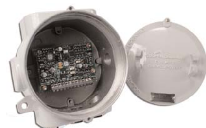
DDM800 Module in EExD Housing
